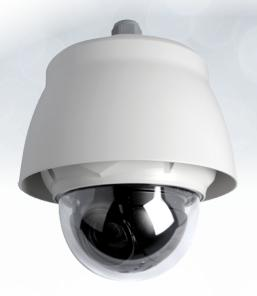
Vicon's Cruiser™ high definition (HD) vandal PTZ dome camera is available in an extreme weather version. This version includes a sunshield and heater/fan electrical components to extend the operating temperature range to -50° to 65° C.
